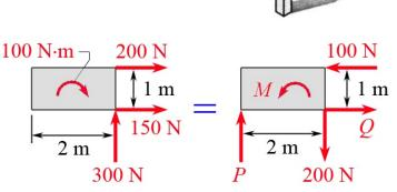
**1.** Applying the *rigid-body principle* ① and the *moment of a couple*,
