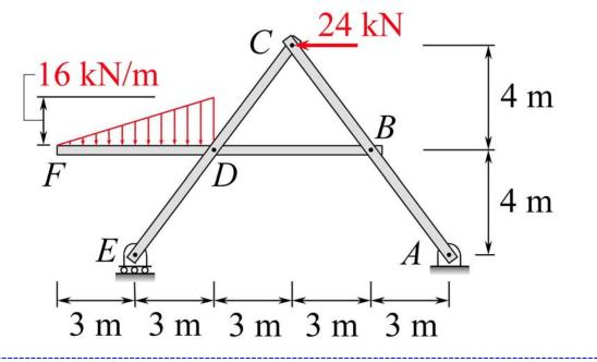
FBD for member ABC with no pins (2) FBD for member BDF (1) FBD for entire frame (1) A = 24i - 12j kN (2) B = -42i + 16j kN (2) C = 18i - 4j kN (2)
