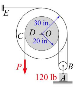
*Hint*. Consider the cases: (a) slipping between belt and drum D is assumed to impend, (b) slipping between belt and drum C is assumed to impend.
