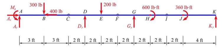
**Step 2:** We draw the *VDD* for the beam with a **strategy** to involve  $M_A$  in the total virtual work done.
