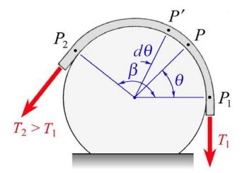
Including a **free-body diagram** of the belt element *PP'* and **definitions** of all symbols used, **derive** the **formula** for a flat belt having an impending slipping around a drum as shown.
