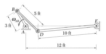
the ground link AE. Determine the value of  $\omega_{AB}$ .
