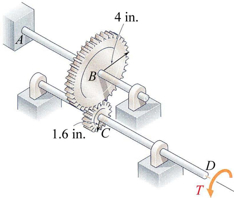
$$T_{CD} = 12 \times 10^3 \text{ lb}\cdot\text{in.} \quad 12 \times 10^3 = 1.6 F \quad F = 7500 \text{ lb} \quad \textcircled{2}$$
