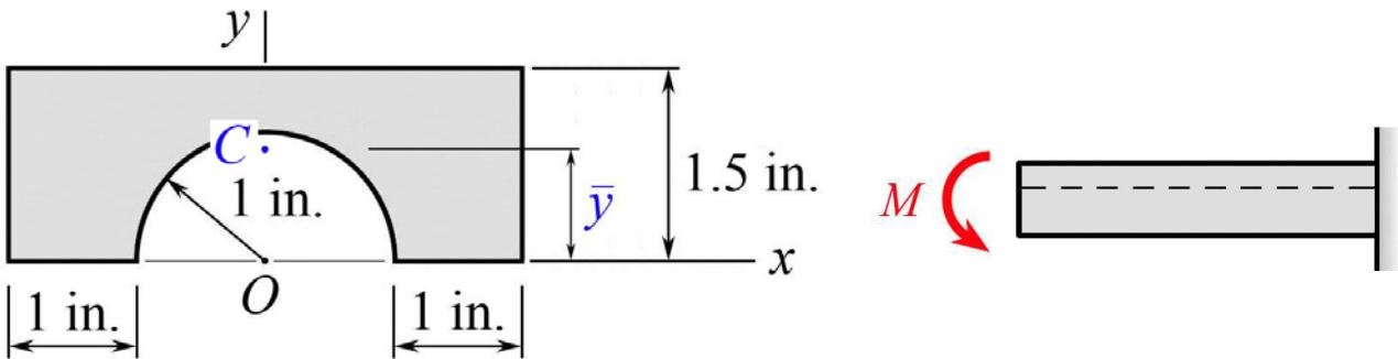
$$(a) A_1 = 6 \text{ in}^2 \quad A_2 = -\pi/2 \text{ in}^2 \quad \bar{y}_1 = 0.75 \text{ in.} \quad \bar{y}_2 = 4/(3\pi) \text{ in.} \quad \textcircled{1}$$
