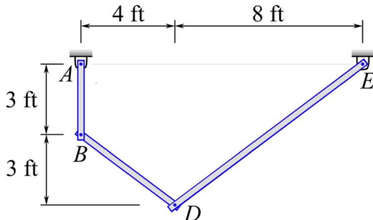
$$(a) \quad \omega_{AB} = 10 \text{ rad/s} \quad \text{③} \quad \omega_{BD} = 5 \text{ rad/s} \quad \text{③}$$
