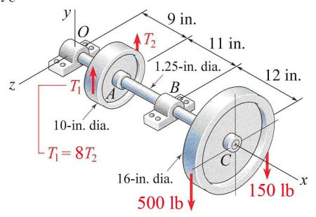
$$E = 30 \times 10^{6} \text{ psi} \qquad I = \frac{\pi}{4} r^{4} \qquad T_{1} = 640 \text{ lb} \qquad T_{2} = 80 \text{ lb} \text{ } \text{ } \text{In}$$
