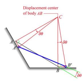
A body undergoes virtual displacement from position AB to position AB'. The **displacement center** is at *C*.
