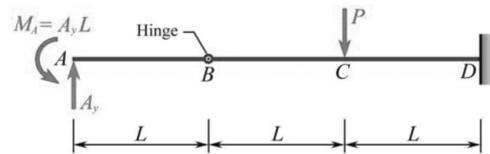
Fig. 3. Reactions at end  $A$  of the beam in Fig. 2.
