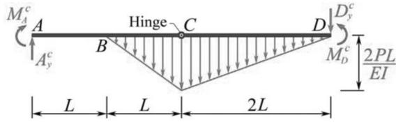
Fig. 8. Free-body diagram for the conjugate beam in Fig. 7.
