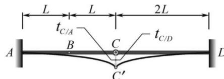
Fig. 10. “Deflection” of the conjugate beam in Figs. 7 and 8.
