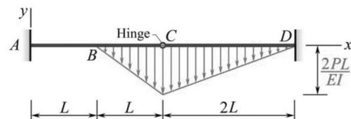
Fig. 7. Conjugate beam for the beam in Fig. 1.
