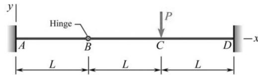
Fig. 2. Statically indeterminate beam with a hinge connection.
