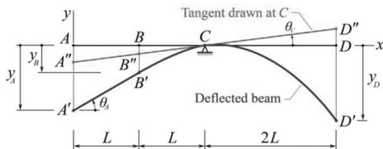
Fig. 11. Obtained configuration of deflections of the beam in Fig. 1
