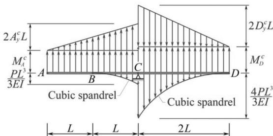
Fig. 9. “Conjugate beam” for the conjugate beam in Figs. 7 and 8.
