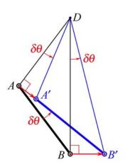
A **compatible virtual displacement** of a member AB is an imaginary displacement resulting from a *first-order* differential angular displacement  $\delta\theta$  of the member about a certain point *D*, called its **displacement center**, during which the member *deflects* from position AB to another position A'B' and the following conditions exist
